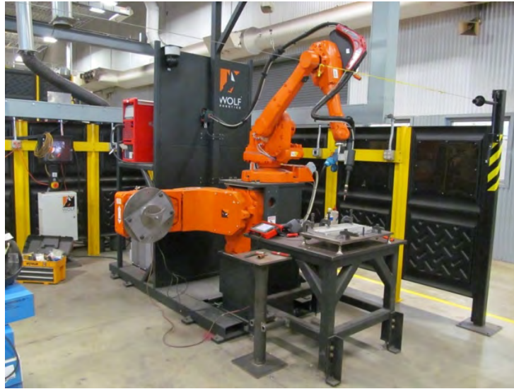
Fig. 1 ABB IRB 1600 Robot and Fronius welding system with push-pull type wire feed system
