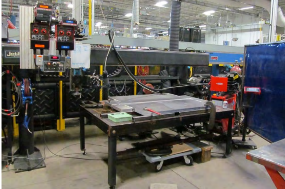
Fig. 5 Tasks 2 and 3 Fronius TPS 5000 weld system, Jetline Engineering side beam, and push-pull wire feed
