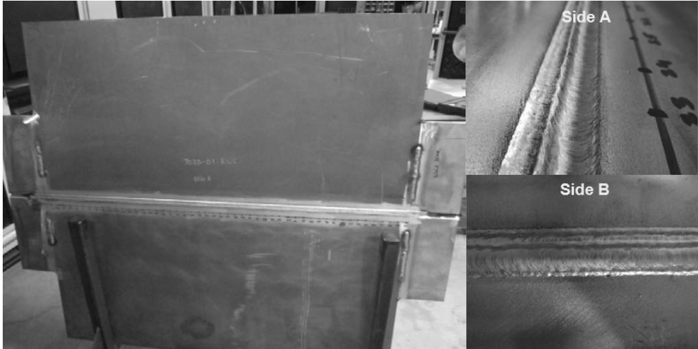
Fig. 26 Photographs of 25.04-mm-thick ballistic panel 7020-01-EWI prior removal of end tabs
