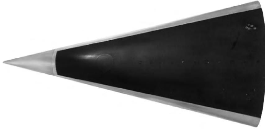
Figure 2: Wind tunnel model, looking down on semi-major axis plane
