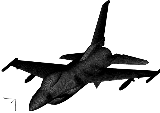
Figure 2: Surface mesh of an F-16 with two under-wing GBU-38 stores placed approximately at the mid-wing pylon stations.
