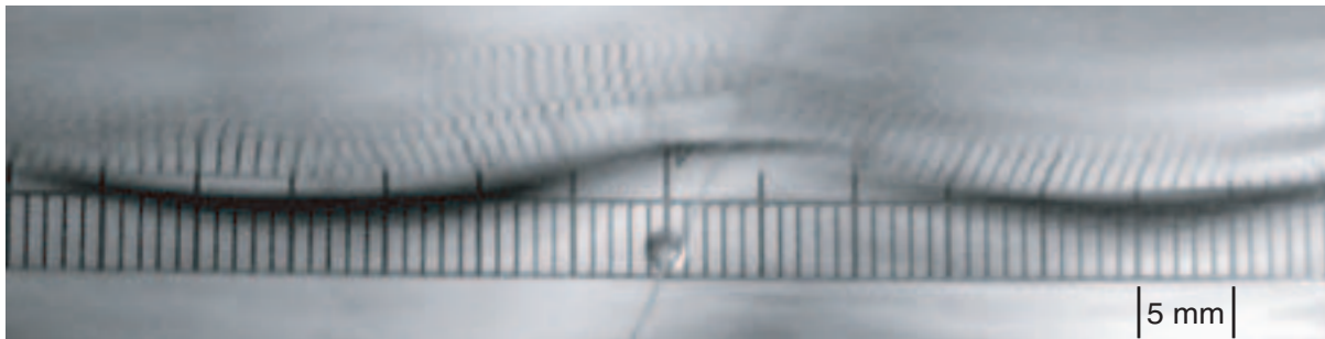
Figure 1. Photograph of a single bubble below a slightly roughened air-water interface and scaled ruler (1 mm graduation). [Figure is for demonstration purposes only, and illustrates how the rough surface was quantified using digital photography. Acoustic measurements were not made while the scaled ruler was in the water.]
