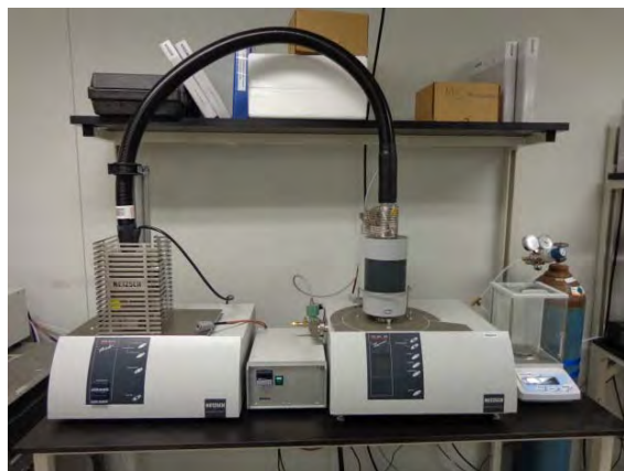
Fig. 4. Left: mass-spectrometer (Netzsch QMS Aeolos); right: differential scanning calorimeter (Netzsch DSC 404 F1 Pegasus).
