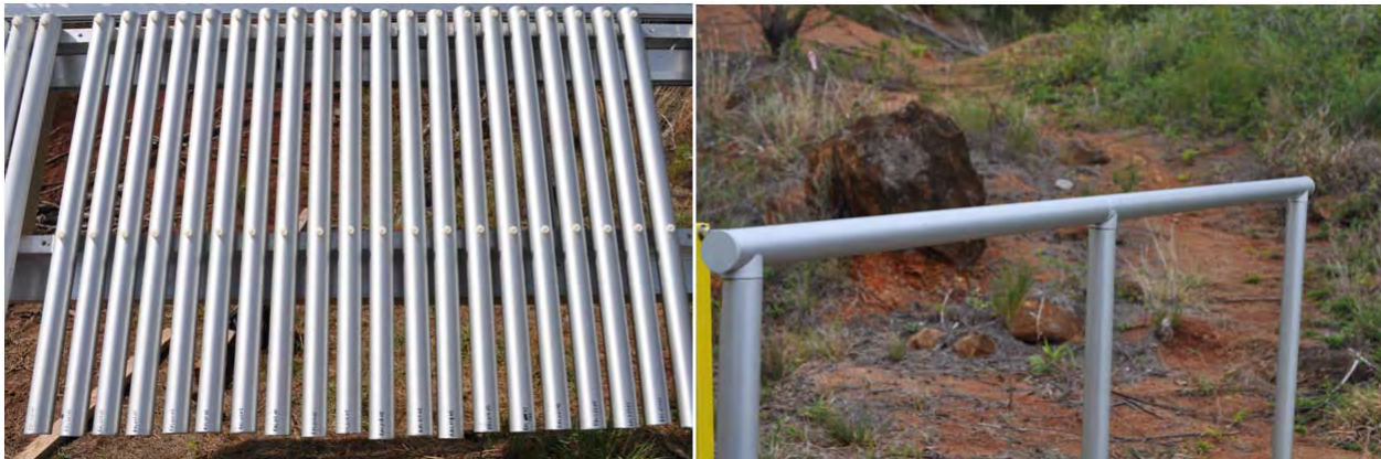
Figure B69. (Left) Aluminum railing coupons. (Right) Aluminum railing test section.
