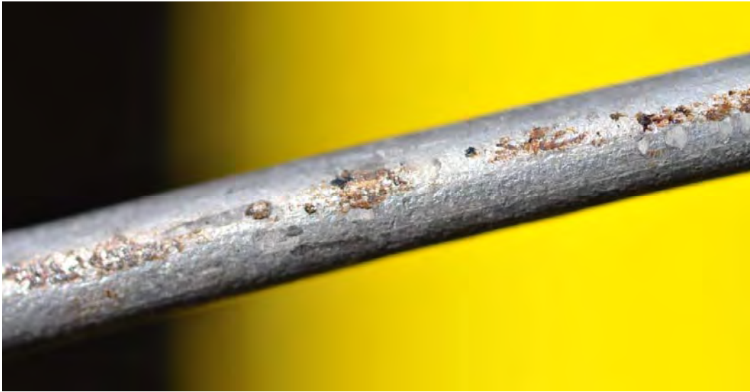
Figure B177. Aluminized Steel Wire Coupon
