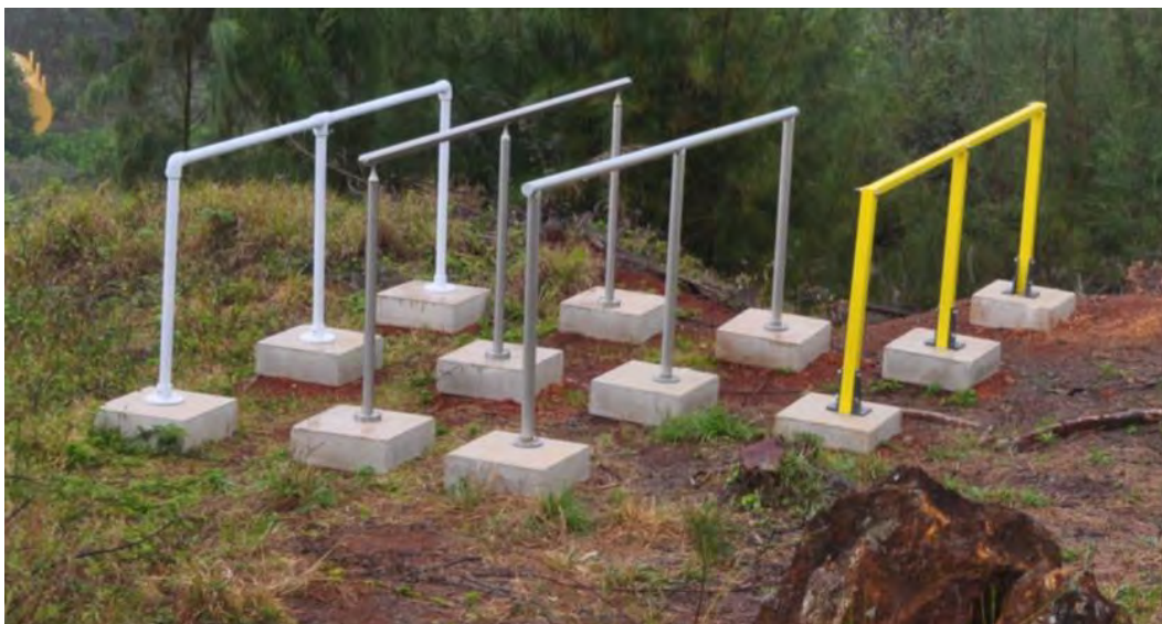
Figure 7. Railing test sections installed at KTA.
