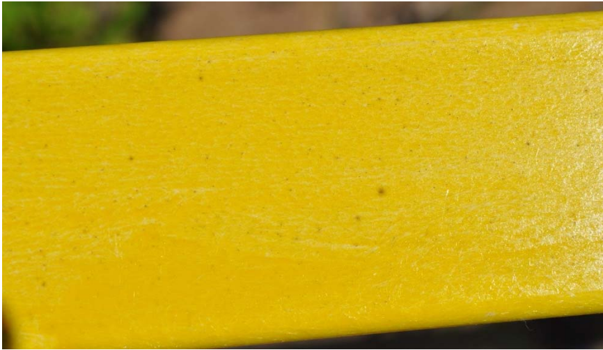
Figure B22. Fabricated FRP Railing
