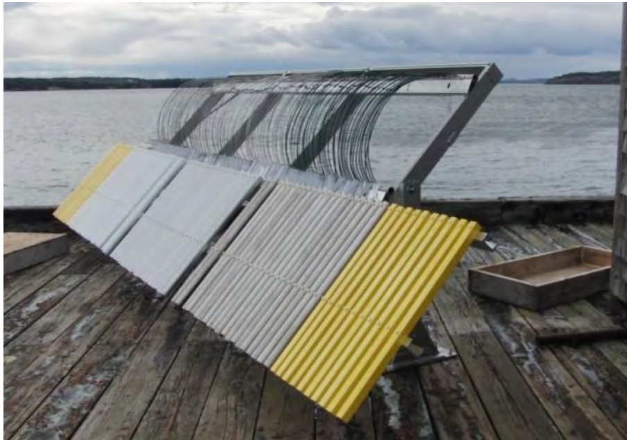
Figure 13. Railing and wire coupons installed on exposure rack placed at 45 degree angle at Treat Island.
