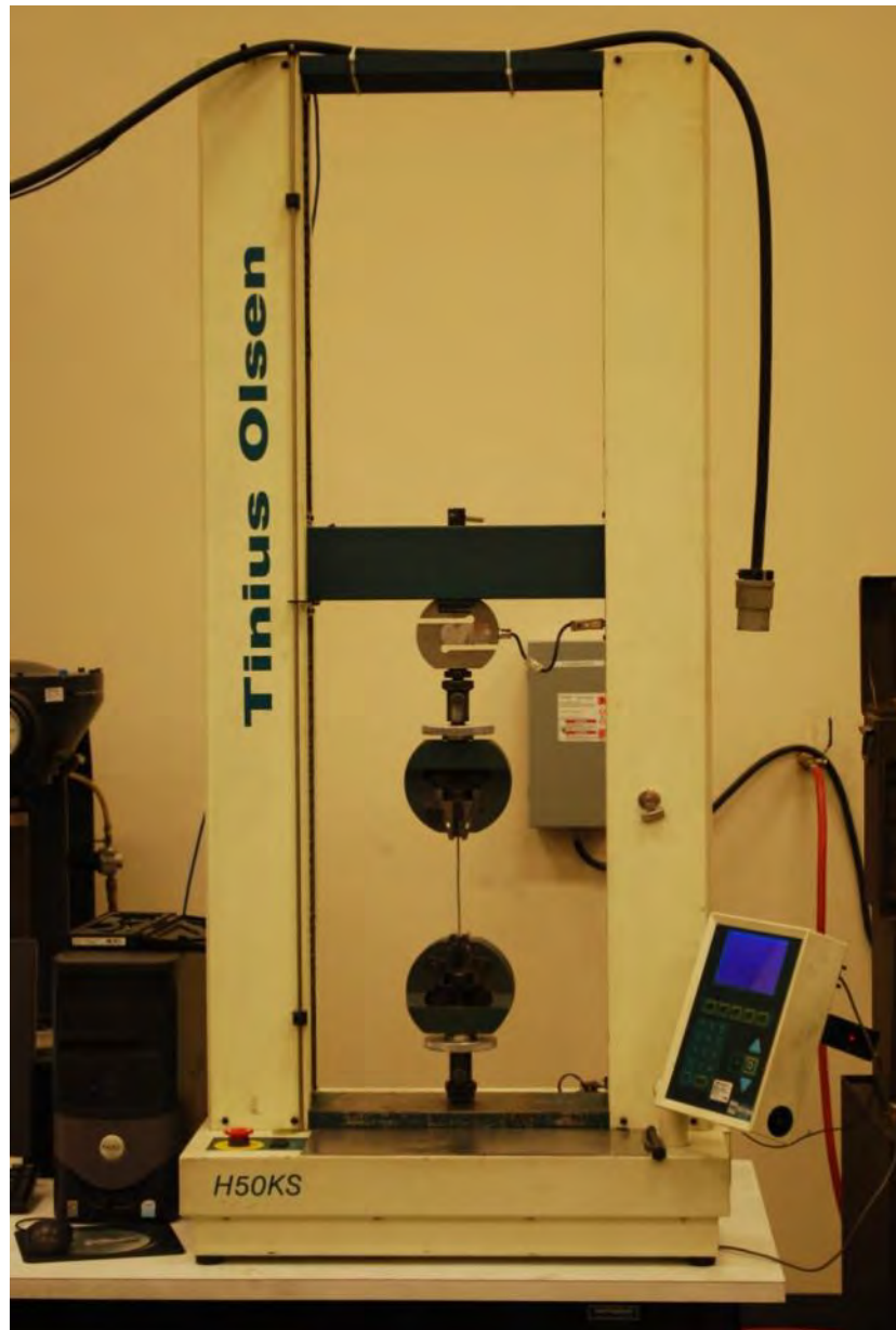
Figure 16. ASTM A931 tensile test of wire coupons after exposure.
