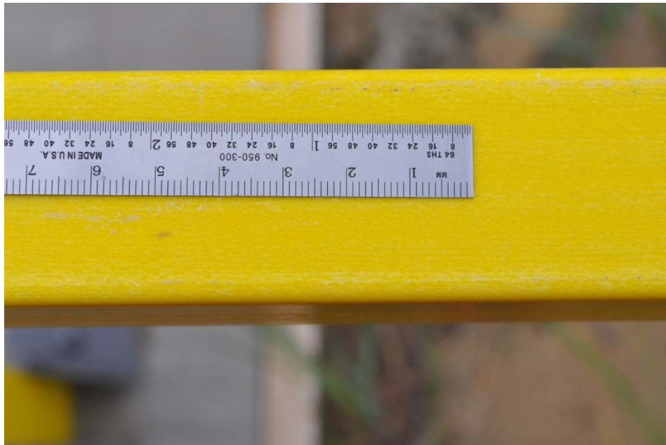
Figure B2. Fabricated FRP Railing
