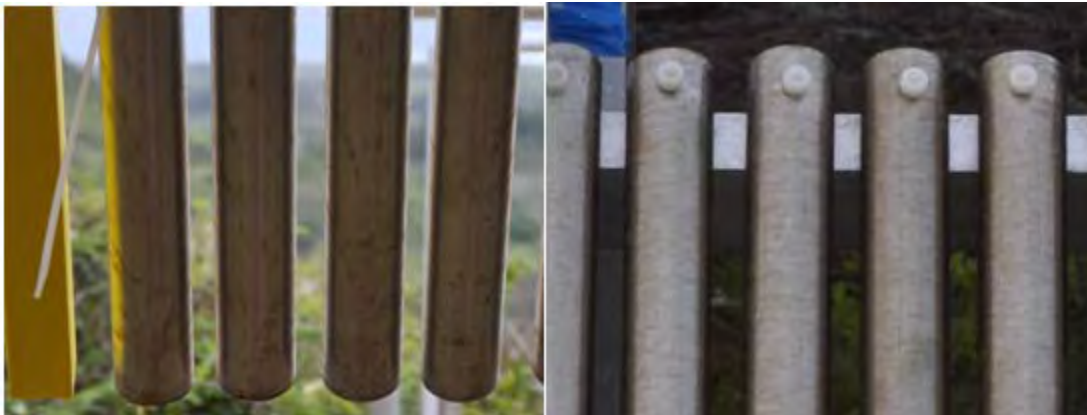
Figure B66. (Left) Stainless steel coupons facing away from the ocean; (Right) stainless steel coupons facing the Ocean.
