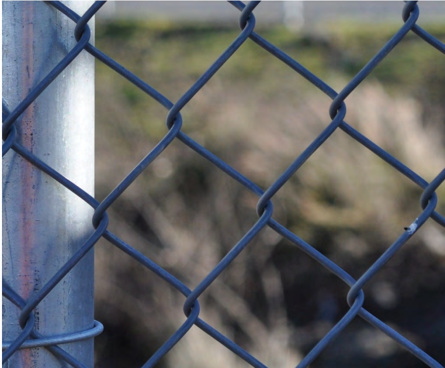
Figure A13. Galvan PVC after 6 months exposure.
