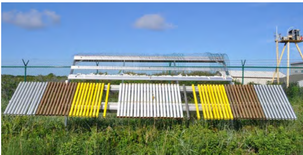
Figure 12. Railing and wire coupons on exposure rack placed at 45 degree angle at the FRF.
