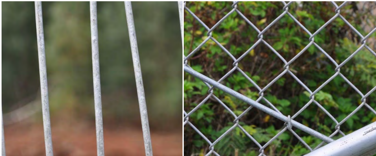
Figure B72. (Left) Aluminized Steel Wire Coupons. (Right) Aluminized Steel fabricated fencing
