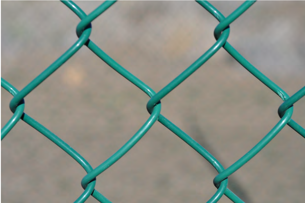
Figure A7. Fuse-bonded PVC after 6 months exposure.
