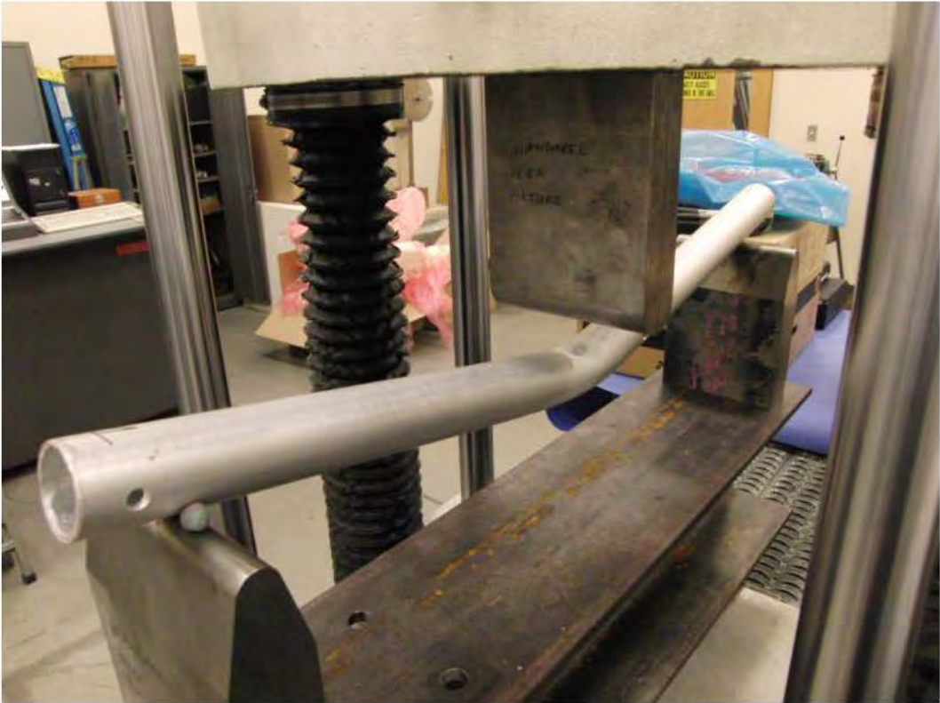
Figure 17. ASTM D790 flexure test of railing coupons after exposure.
