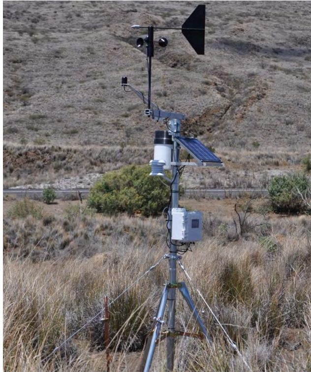
Figure A6. Weather station.
