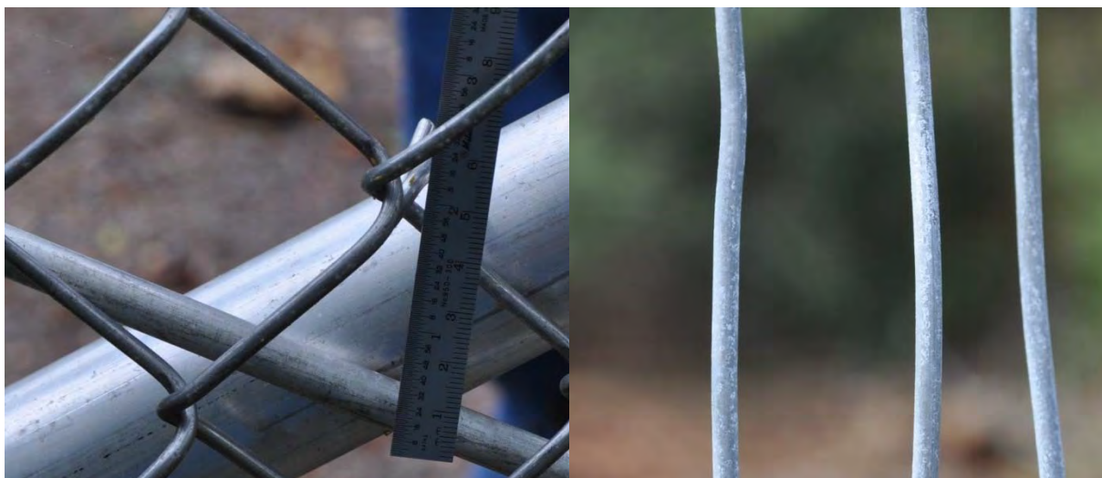
Figure B73. (Left) Galfan fabricated fencing. (Right) Galfan Wire Coupons
