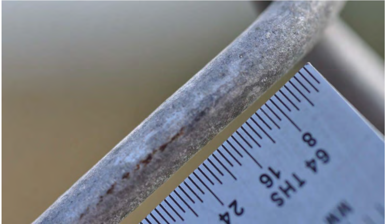
Figure B108. Aluminized Steel Wire Fencing
