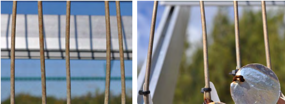
Figure 20. Stainless steel wire coupon at FRF (left) and KTA (right) after 6 months of exposure.
