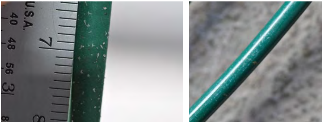
Figure 22. Standard PVC coated galvanized steel wire coupon at FRF (left) and KTA (right) after 12 months of exposure.
