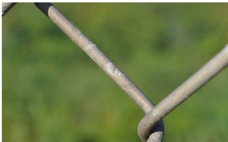
Figure B32. Aluminized Steel Wire Fencing
