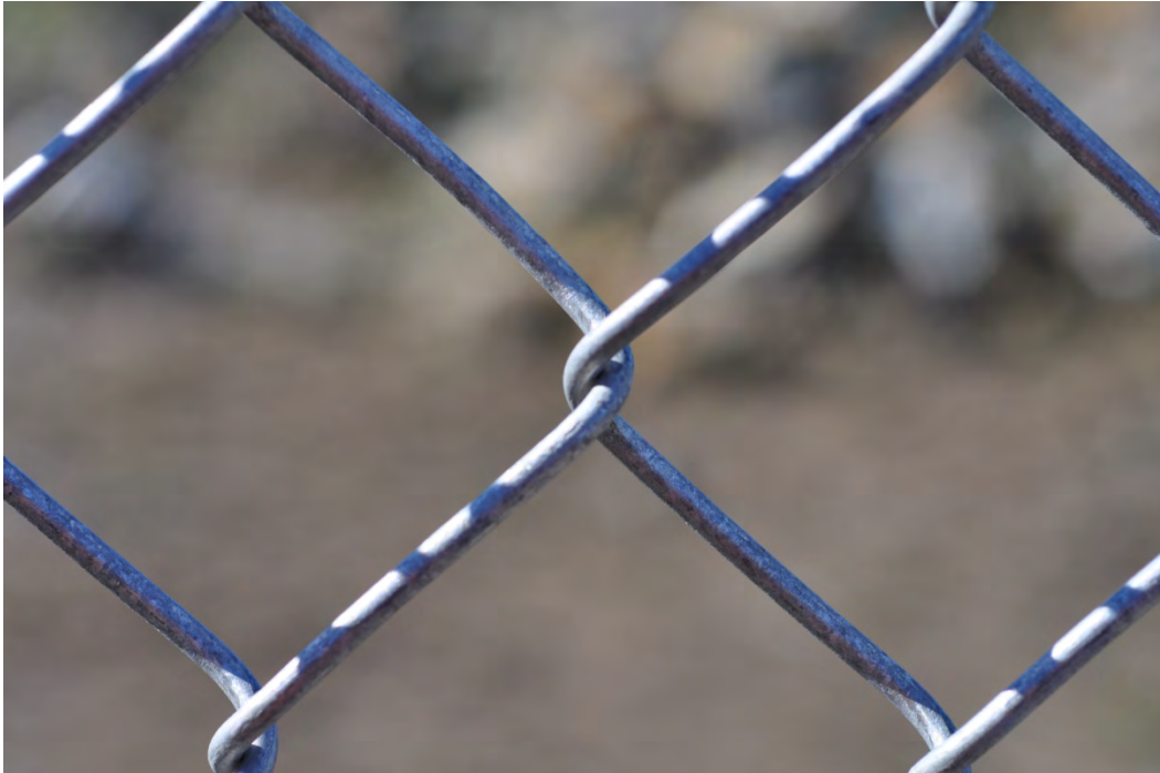
Figure A11. Aluminized after 6 months exposure.
