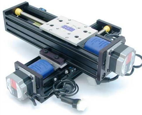
Figure 3. Linear actuator assembly. Velmex ® BiSlides ® (pictured with Velmex ® motors) are attached orthogonally such that the base of one is mounted on top of the plate of the second. The x- and y-axes are coupled in this way in the system design, and the z-axis stands alone.
