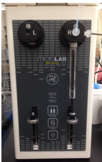
Figure 7. Syringe pump. Hamilton ® Microlab ® 625. The left side is empty, but the right side is loaded with a glass syringe. Movement of the plunger draws in solution from the tubing entering the side of the valve, and dispenses solution out the tubing from the front of the valve.
