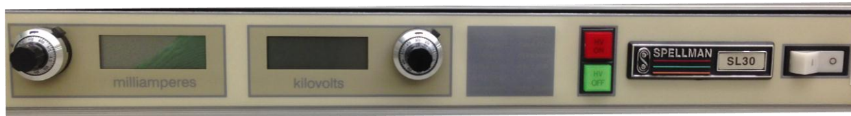
Figure 8. High voltage power supply. Spellman ® SL Series. Current and voltage controls and indicators appear on the left. On the right, a rocker switch turns power on. As a safety measure, the power supply will not output a set voltage until the red HV ON button is pressed.
