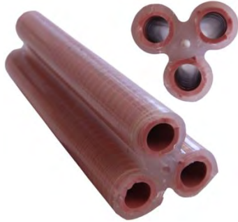
Figure 21. Multi-DOF bending actuator consisting of three fiber reinforced linear actuators co-molded together.
