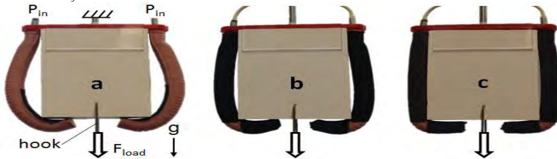
Figure 19. The proposed sleeve method enables improved shape matching to angular objects and holding strength.
