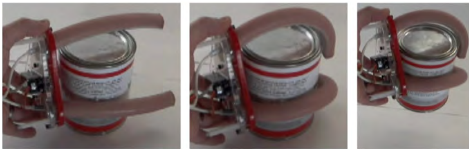
Figure 26. All fingers are activated to conform around and pick up a quart sized metal can.
