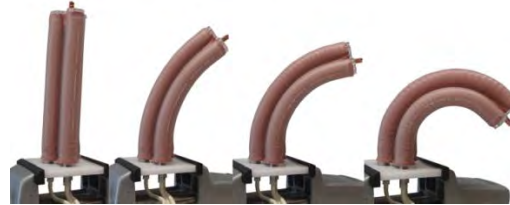
Figure 22. Gradual pressurization of one of three chambers.
