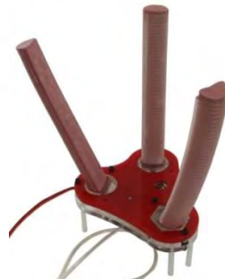
Figure 24. Soft Actuated version of i-HY Hand
