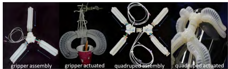
Figure 35. (left to right) Three modules assembled into a three port soft manifold to form a gripper – shown picking up a paper cup. Then four modules joined to two manifolds, where the two manifolds are similarly joined together – the final form is that of a quadruped.
