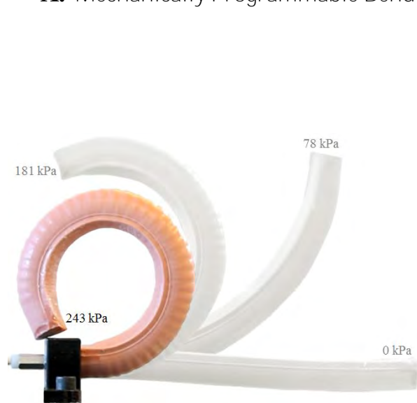
Figure 12. Range of motion of the fiber reinforced soft bending actuator constructed from 28A durometer rubber (see Table I for material properties).
