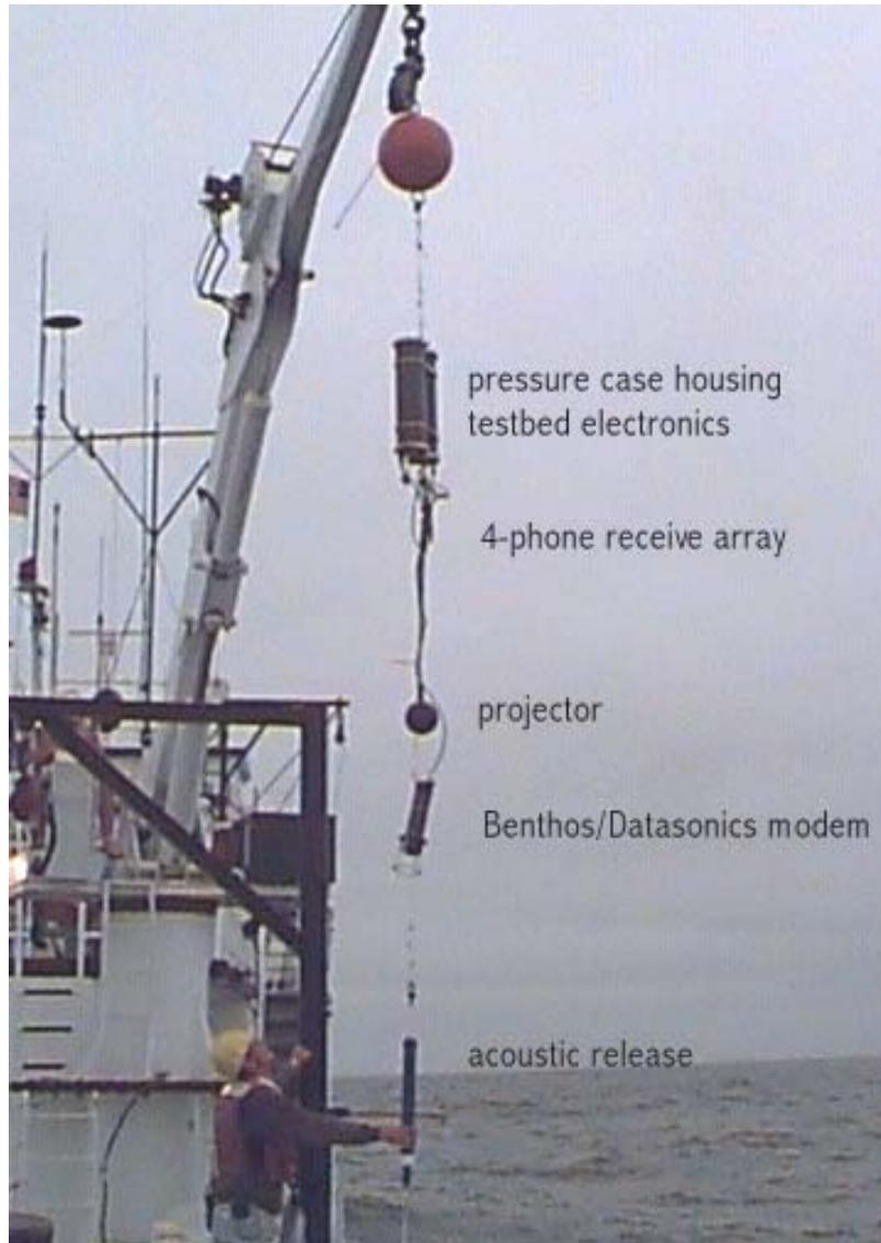
***Fig. 1: Testbed configuration.***
