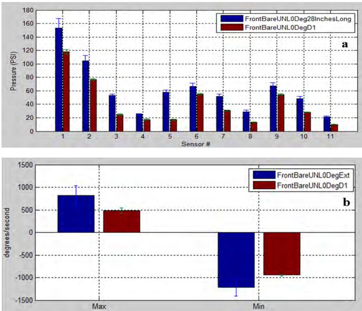
Figure 24. Comparisons of (a) overpressure, (b) angular velocity for a front facing bare head inside a 28” shock tube and outside at distance D1 in 9” shock tube.
