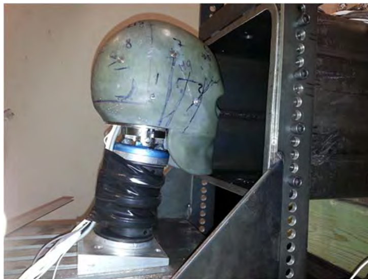
Figure 3: Picture showing that the RED head was placed outside the 9" shock tube. The RED head nose tip was 1.5" from the tube muzzle and centered with the tube center line and in 0° position using the NATICK manufactured wedge base.
