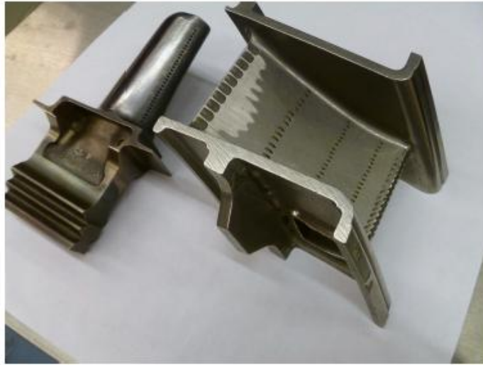
Figure 1: Superalloy turbine blade with cooling ports, reproduced from Shillig [9]
