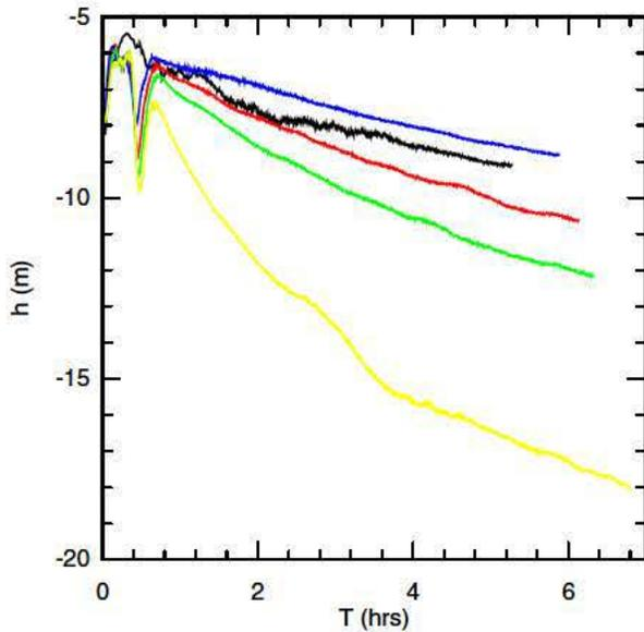
Figure 5: Variation of ocean mixed layer depth with time for varying stratification  $N$ . All runs have  $La_t = 0.5$  except for the black line which has  $La_t = \infty$  (no wave effects).  $N = [2.2, 1.4, 1.4, 1.0, 0.44] \cdot 10^{-2} \text{ s}^{-1}$  for [blue, black, red, green, yellow] lines, respectively.
