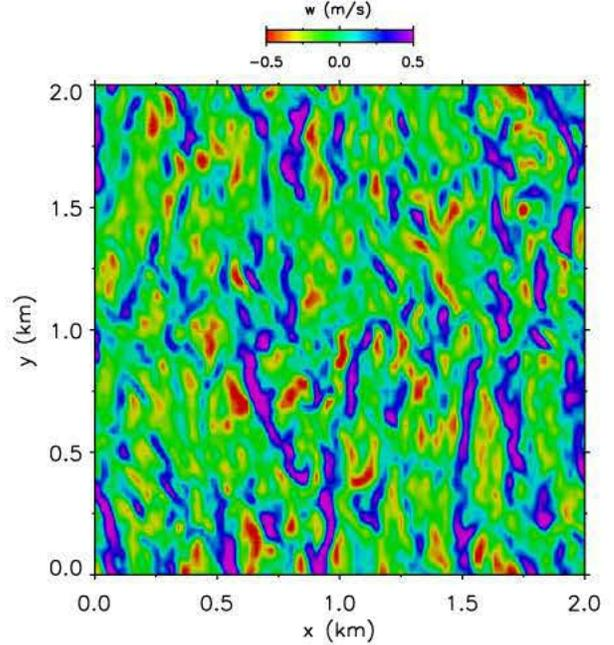
Figure 4: Snapshot of the vertical velocity field at  $z = 25$  meters above the surface at  $t = 7.6$  hrs with  $z_i/L = -10$ . Streaky patterns aligned with the surface winds are the dominant coherent structure.
