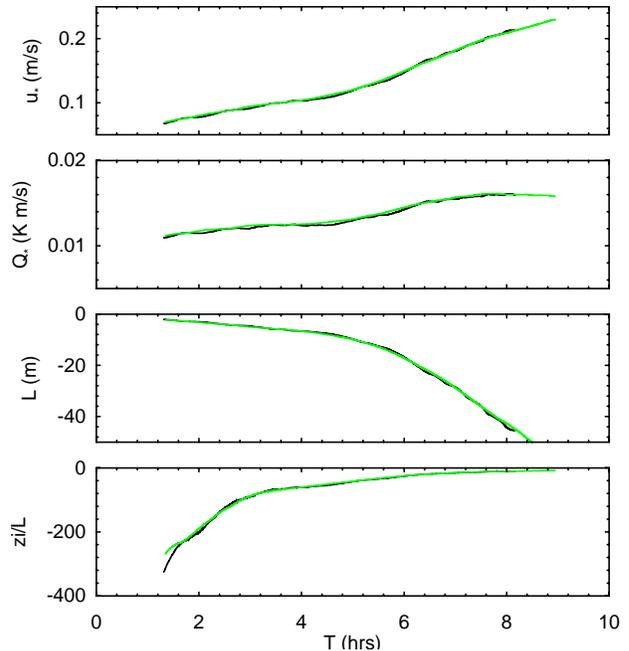
**Figure 2:** Friction velocity  $u_*$ , surface heat flux  $q_*$ , Monin-Obukov length  $L$ , and stability parameter  $z_i/L$  at the CBLAST low-wind site. Black and green curves correspond to small and large horizontal LES domains.
