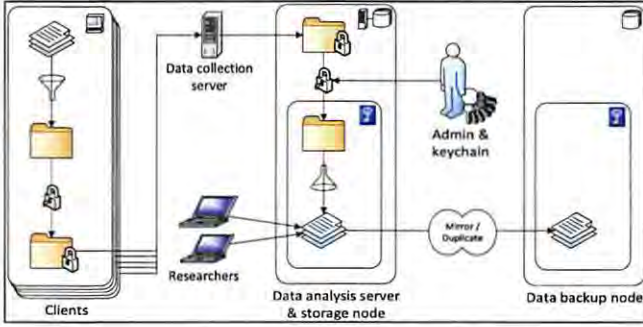
Fig. 2. Our SBO high-level hardware architecture and data flow.
