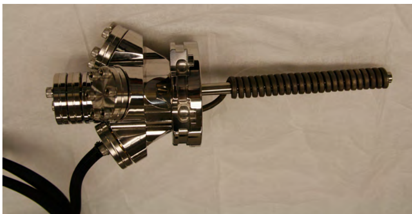
Figure 5.6: Picture of the directional doser with heating coil.
