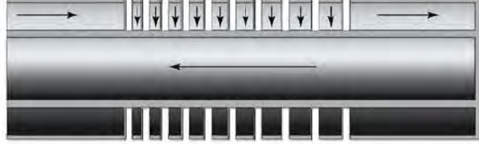
Fig. 2 The helical section replaced by discrete rings of current
