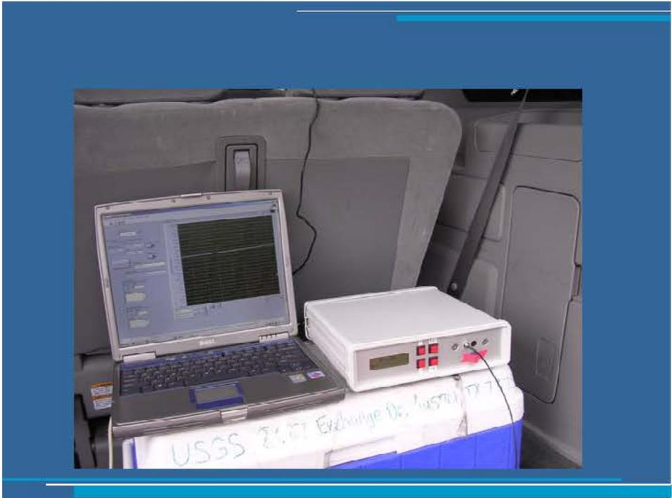
Figure 4-8. Flow-through cell readout setup.
