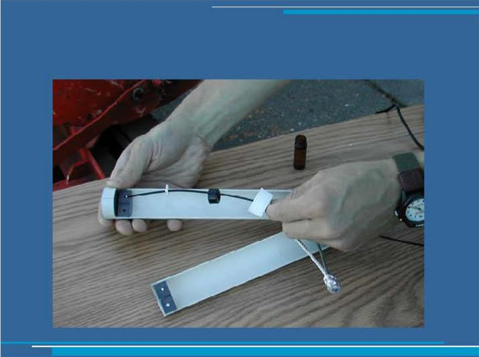
Figure 4-12. Down-hole profiling setup.
