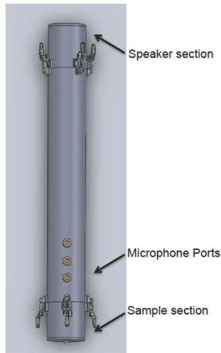
Figure 3.1: The vertical impedance tube is shown has three sections. The top section holds a speaker that introduces sound into the next section which is hollow and has three ports for 1/2" microphones near the sample section. Ten identical simple sections were constructed for this study so that samples could be prepared and tested without disturbing their structure.
