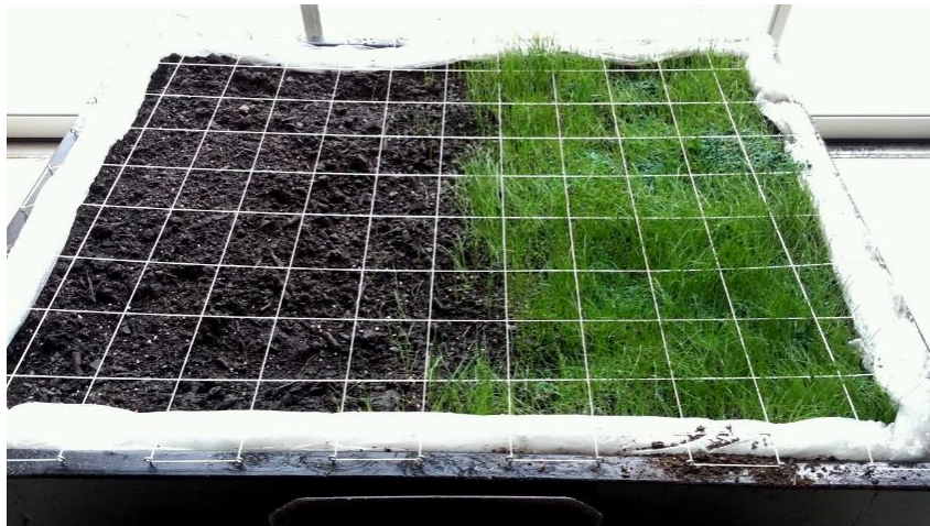
Figure 4.1: The sample grow box is show. On the right side is germinated kentucky perennial grass. On the left side soil that has been sieved to 4.75 mm grain size. The 4 inch grid system marks each sample to be cut
