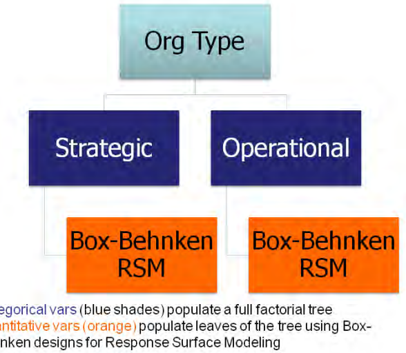
Figure 123: Graphical rendering of experimental setup with factor tree and Box-Behnken leaves
