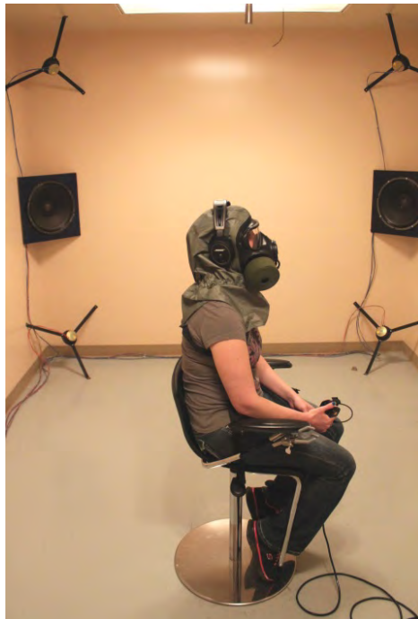
Figure 5. Subject completing the threshold measurement with the JSAM-SA and a communication headset
