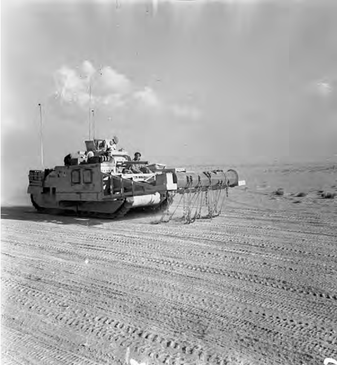
Photograph of Scorpion Mine-clearance Device Affixed to Tanks
