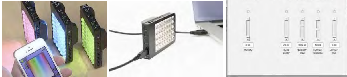
Figure 5. The KICK light device contains a LED panel that can produce different colors of light at different intensities, and can be controlled wirelessly from a smartphone app (picture on left), or through an SDK from a laptop or desktop device (middle picture). We have developed a Matlab GUI (picture on right) to control the KICK light from a desktop PC.
