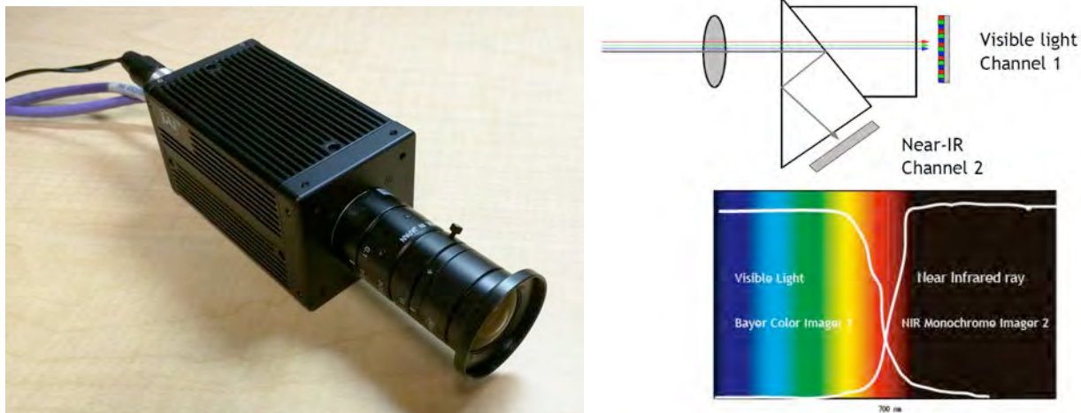
Figure 3. The JAI AD-130GE camera (left) combines both a color video sensor and an infrared video sensor mounted on the same optical axis (right), enabling one to easily locate and compare the image parameters of different facial features as seen in both the visual and infrared spectra. For example, the contrast at the pupil border between the a blue iris and the pupil is low in the infrared spectrum, but significantly higher in the visible spectrum.
