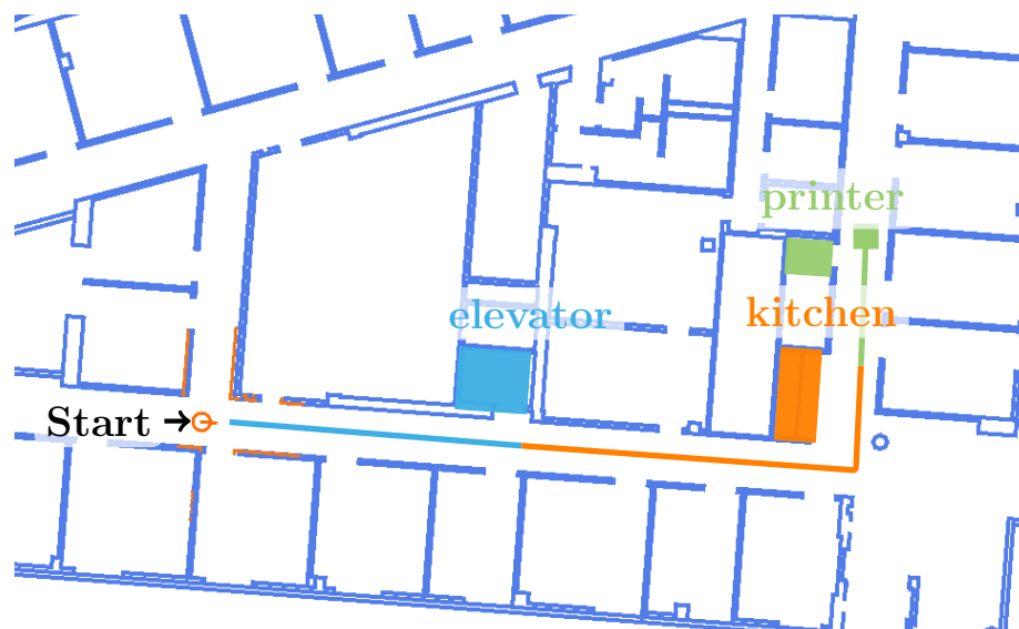
Figure 7.3: Trace of successful CoBot run for following the command “go towards the elevator, turn left towards the kitchen, and go towards the printer.” We show the complete robot’s path through the world (color-coded by SDC), as well as the landmarks the policy used to follow the direction. Note that we show the entire environment, but CoBot only had access to the parts of the environment it had visited (a partial map).
