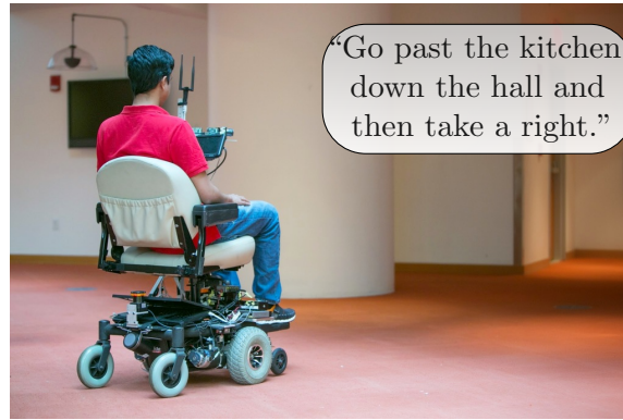
Figure 5.1: One possible natural language command for an autonomous wheelchair. Since the user may be able to see beyond the robot’s perception range, they may be able to communicate information about the world and the desired task through a single natural language command.
