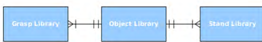
Figure 24. Relationship between objects, grasps and stand poses libraries using Crow's foot notation
