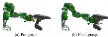
Fig. 2: Using a “ghost robot” the pre-grasp and final-grasp poses (here shown for the drill template) can be visualized prior to perform an arm motion on the real robot.
