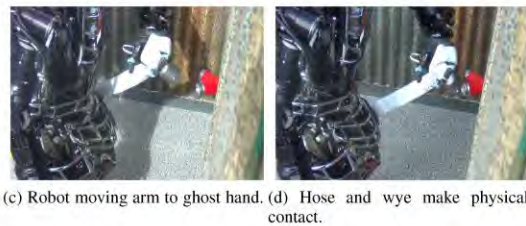
Fig. 11: Robot commanded to bring the hand near the wye and then touch it.
