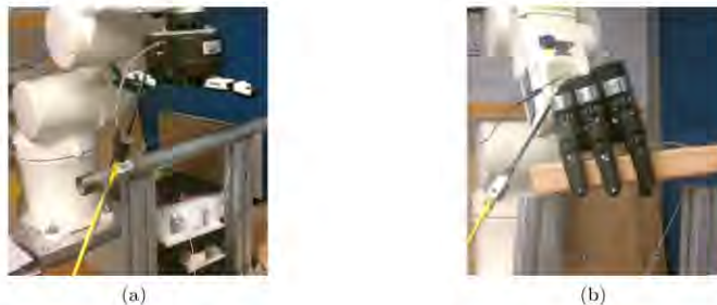
Figure 18: Testing setup with object anchored to table by a cable and force sensor. (a) iRobot hand (b) Sandia hand
