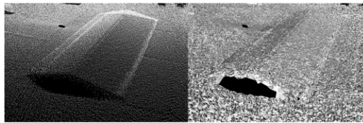
(a) Noisy point cloud and 3D surface reconstruction due to missing filtering
