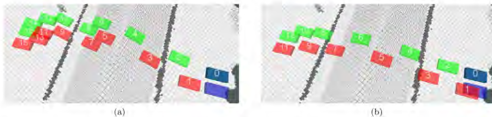
Figure 14: Comparison of different collision check approaches: (a) Occupancy Grid Map (b) Ground Contact Estimation
