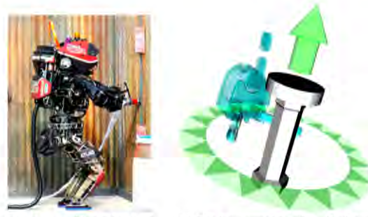
Fig. 1: a) Developed by Boston Dynamics Inc. (BDI) the Atlas robot has 28 hydraulically actuated DOF, weighs approximately 150 Kg and stands 1.88 m tall is shown attaching a fire hose during the DRC Trials 2013. b) Shows the fire hose template, the potential grasp pose of the hand in translucent blue and in translucent green the available affordances of the fire hose, like the circular motion needed to tangle the threads while turning it and the Cartesian translation needed to push the fire hose against the pipe.
