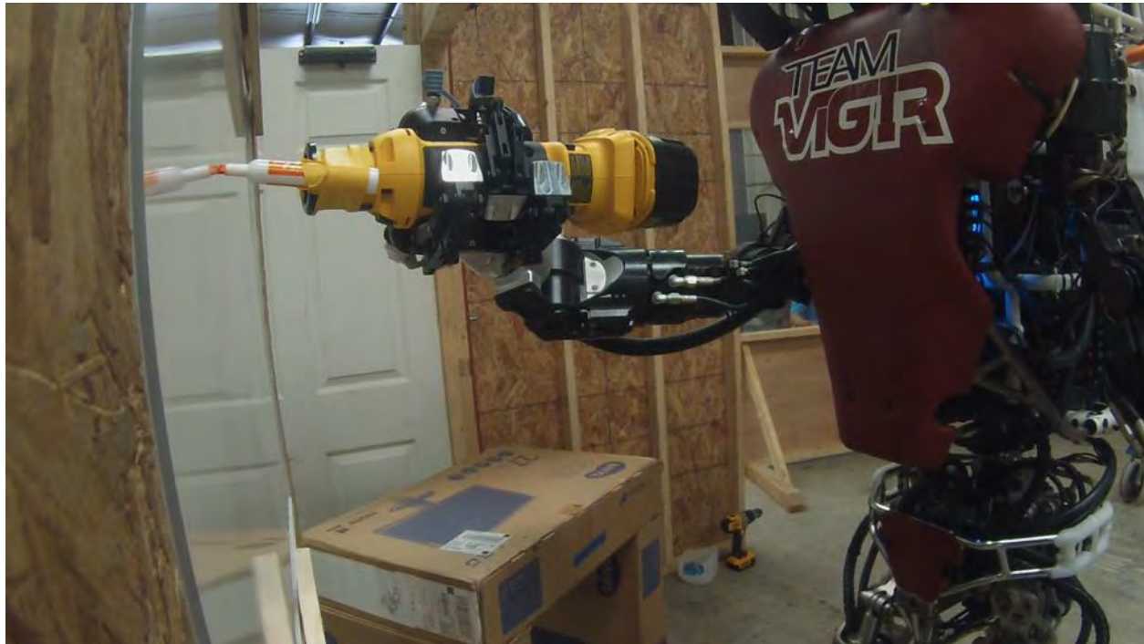
Figure 105. The behavior then moves the cutting tool to a pose in front of the wall
