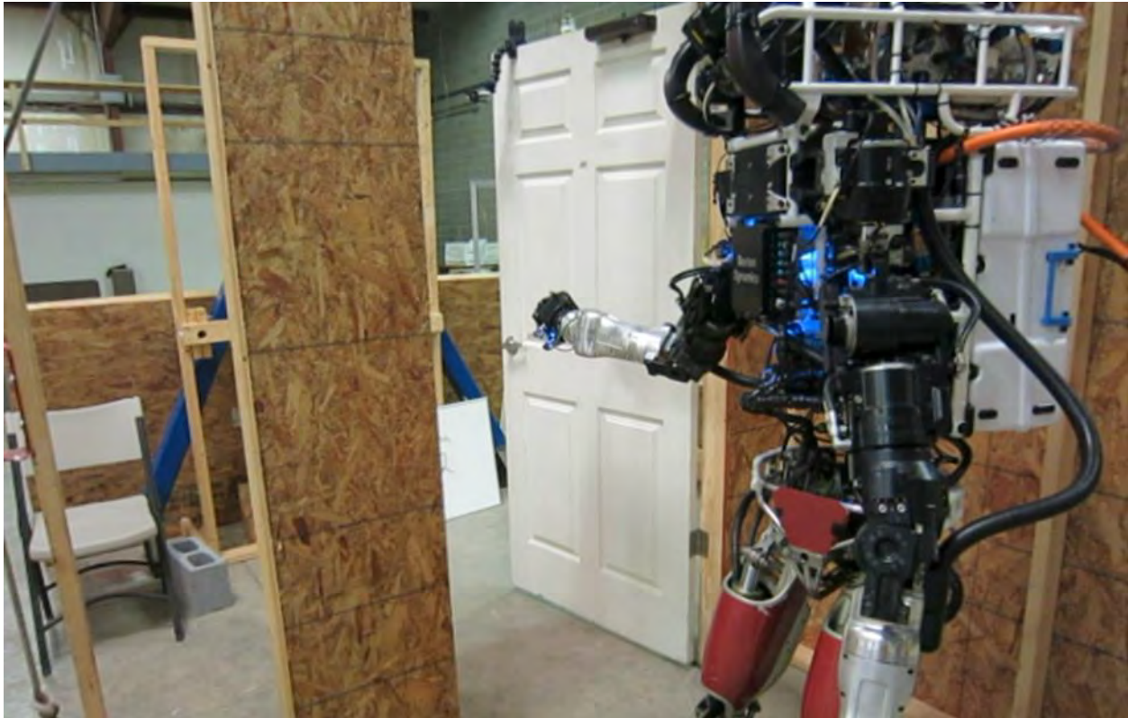
Figure 91. With the door unlatched, the behavior pushes the door completely open.
