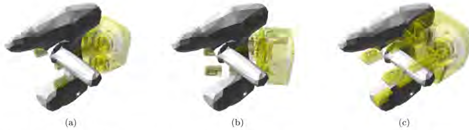
Figure 16: Precomputed Grasps visualized relative to drill template: (a) Front grasp. (b) 45 degrees grasp. (c) Handle grasp.
