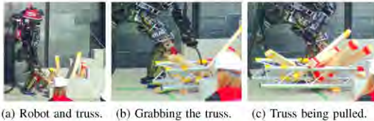
Fig. 9: A door blocked by a truss needs to be pulled away. Utilizing a translation affordance originally designed for an object with translation constraints (e.g. a drawer) can achieve the necessary manipulation motions to pull the truss in a direction parallel to the floor.
