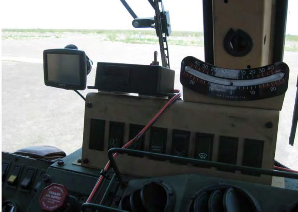
Figure 6. Cab Mounted GPS and Route Timer
