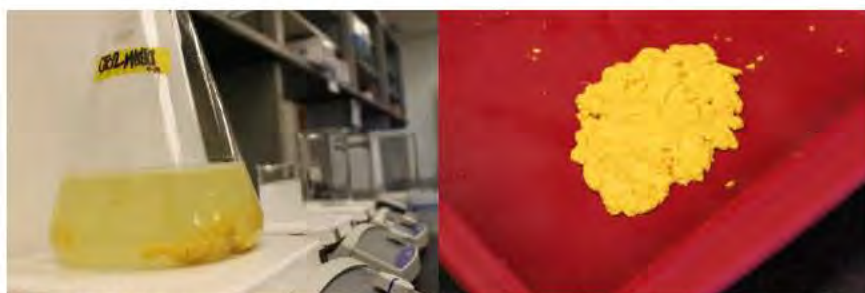
Figure 15. Algal biomass in process of being flocculated and ready for drying oven.
