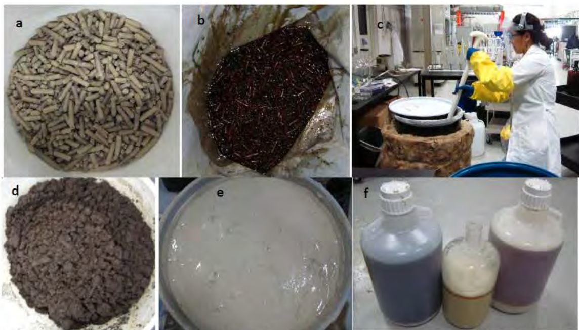
Figure 13. Photos of various hydrolysis process steps including a) pelletized switchgrass feed, b) decrystallization solution, c) hydrolysis step, d) lignin after separation from acidic hydrolyzate, e) gypsum after separation from neutralized hydrolyzate, and f)
