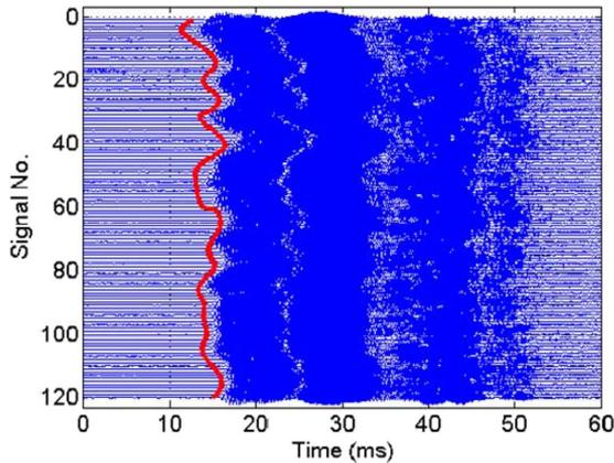
Fig. 11. Calibration data for 120 consecutive transmissions, depth 25 m. Raw LFM signals without pulse compression. Superimposed heavy line shows source-receiver range derived from gyroscope and GPS data and used to correct relative motion.
