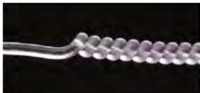
Polymer muscles used to quickly lift and lower a heavy weight (Marcio)
