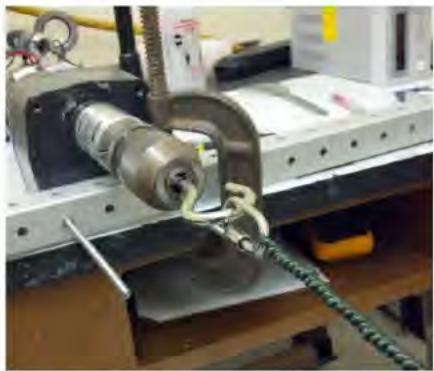
52 coiled, 65 lb test green-dyed polyethylene fishing lines provided the muscle, which was powered by alternating hot and cold water.
