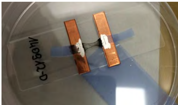
Figure 11. The laser process makes the material transparent and this is likely because it is much less dense. Provided the conductivity also improves, thin and flexible touch screens may be an application.
