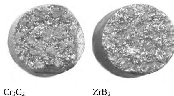
Fig. 1.18. Fracture on a zone of diffusion interaction between \text{ZrB}_2 and \text{Cr}_3\text{C}_2 at 1740^\circ\text{C} .
