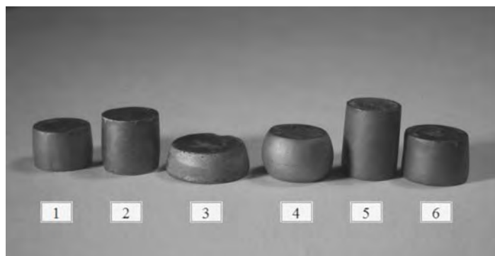
Fig.1.42 Creep kinetics of samples [95%mass.(80% vol. \text{ZrB}_2 + 20% vol.SiC)+5%mass. \text{Cr}_3\text{C}_2 ]
