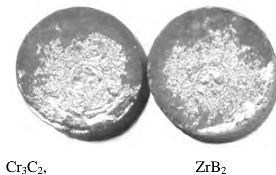
Fig. 1.16. Contact interaction and melting of pair \text{ZrB}_2/\text{Cr}_3\text{C}_2 , temperature 1400^\circ\text{C} , holding - 15 min. A fracture on a zone of contact interaction
