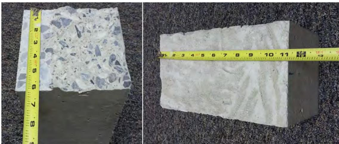
Figure 4-20. The concrete block used for the experiment. The dimensions of the concrete block are measured in inches.
