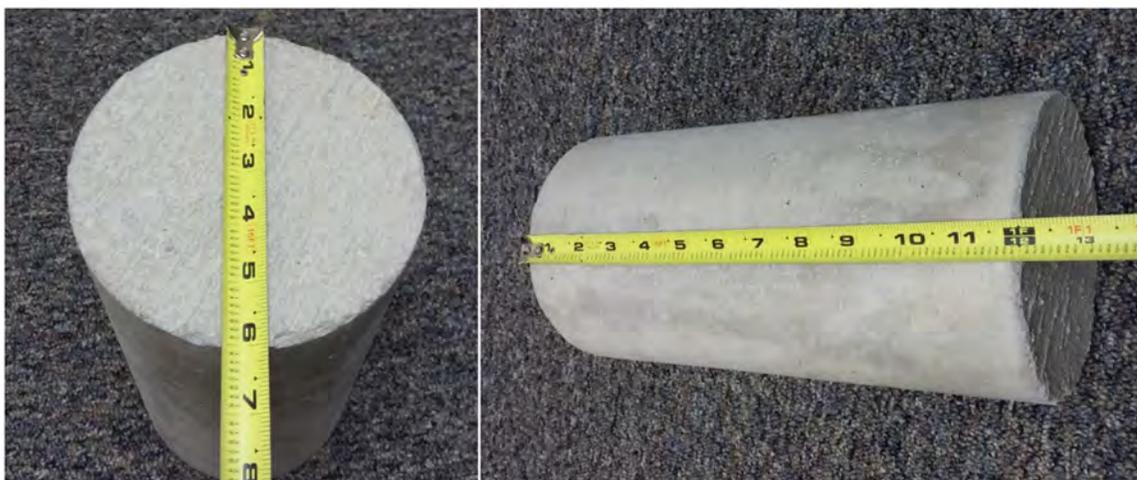
Figure 4-17. The concrete cylinder used for the experiment. The dimensions of the cylinder are measured in inches.
