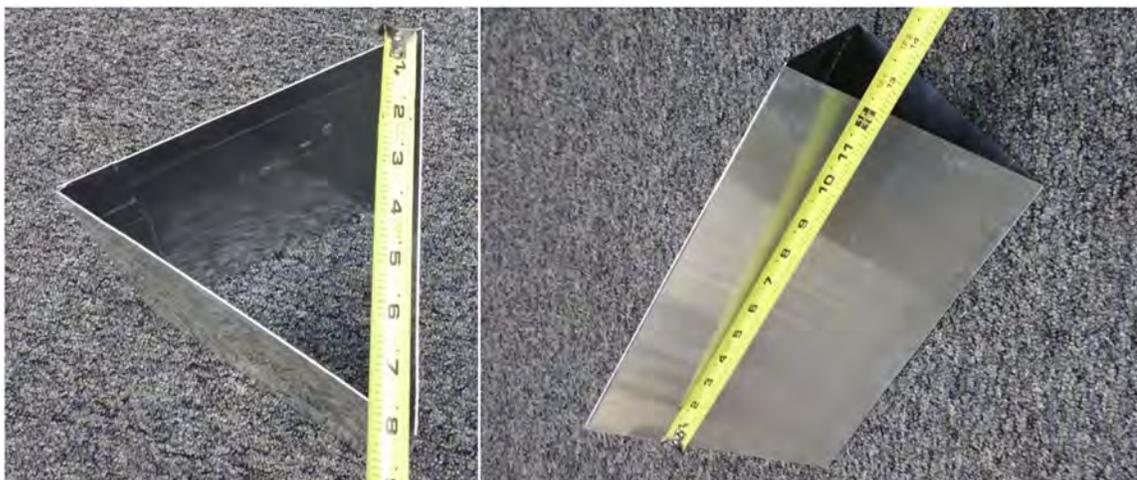
Figure 4-14. The metallic prism used for the experiment. The dimensions of the prism are measured in inches.
