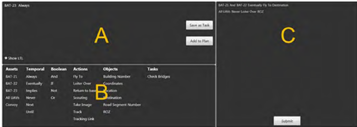
Figure 3. The translator interface and its three windows. A) the proposition editor, B) the token bank, C) the current specification list.
