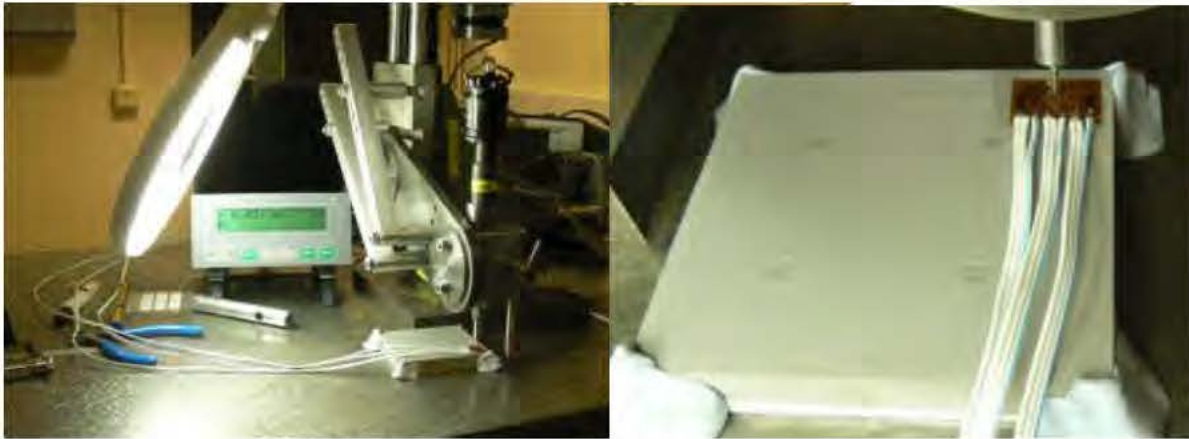
Figure 2-8: Experimental setup for hole drilling measurement
