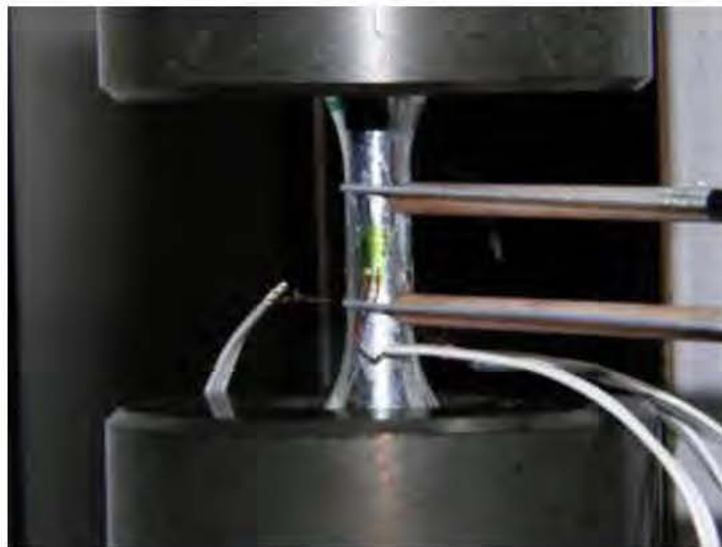
Figure 2-5: Experimental setup for cyclic stress strain test
