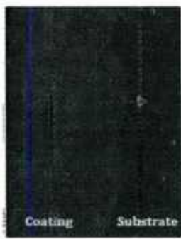
Figure 47. The EDS line scan above across the coating (450°C, 49bar offset: 26mm) and substrate interface does not show any increase in oxygen concentration indicating good bonding.
