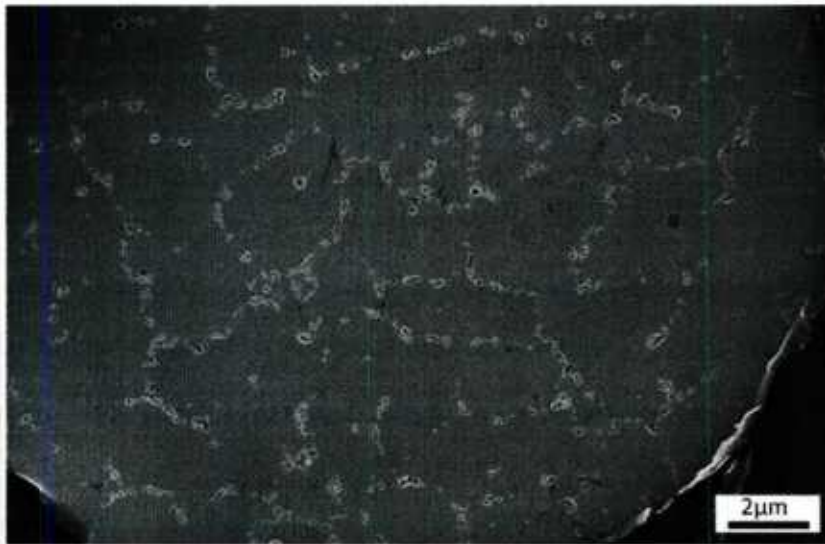
Figure 84. The sensitized 5083 powder had equiaxed grains as revealed with phosphoric acid etching.
