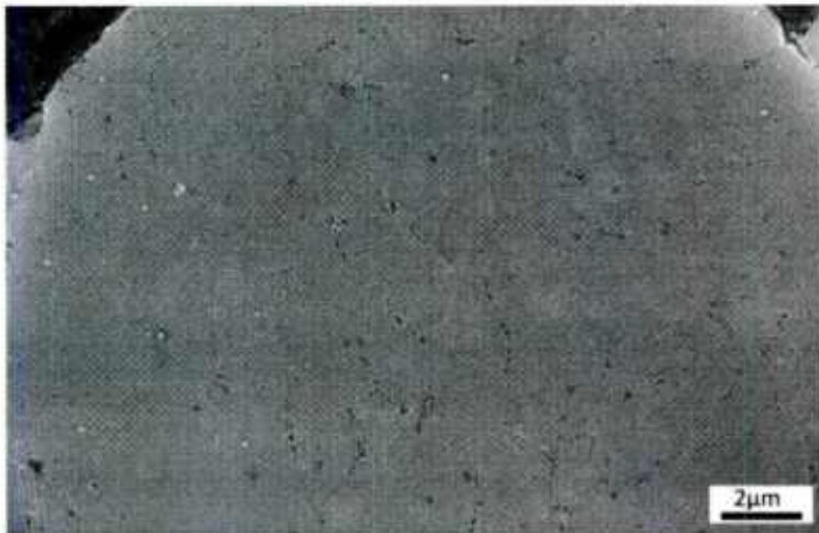
Figure 86. The as-received unsensitized powder also had equiaxed grains though not as distinct compared to the sensitized powder.
