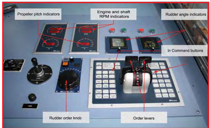
A vessel's engine control station features two identical arrays to control the two propellers. On either side of the order levers are 18 push buttons, 11 of which have assigned functions. These pushbuttons are identical in shape, color, and lettering, and each has a red LED in the upper left corner that illuminates according to functional status. The identical color, luminosity, and size may confuse users. Image courtesy of the United Kingdom's Department of Transportation Marine Accident Investigation Branch.
