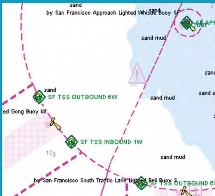
Virtual and synthetic AIS ATONs in an offshore application. Image courtesy of Transas.
