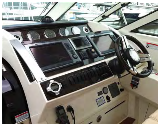
Can "smart boats" be far off? Today, glass helms with multifunction displays offer touch screen control and monitoring.
