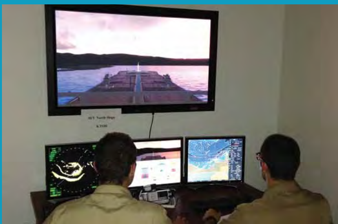
Training for 21 st century waterways will build off of ECDIS training that includes integrating many watchstanding components such as the visual lookout with radar navigation skills. Photo courtesy of the author.
