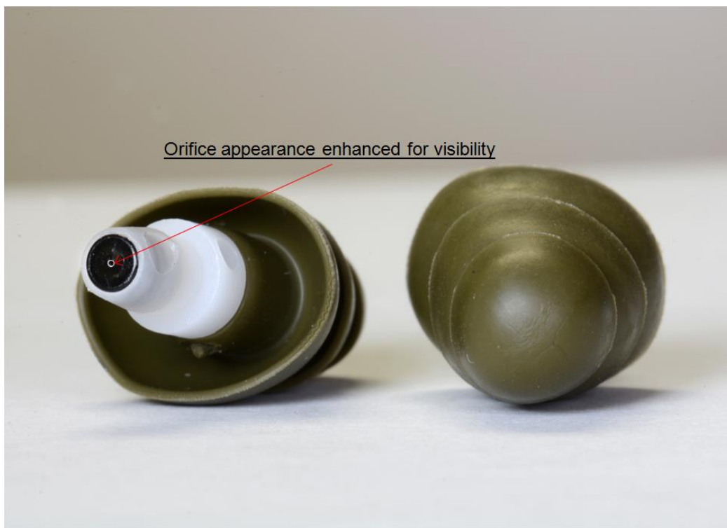
Fig. 5 Dual-ended combat arms earplug; showing open orifice
