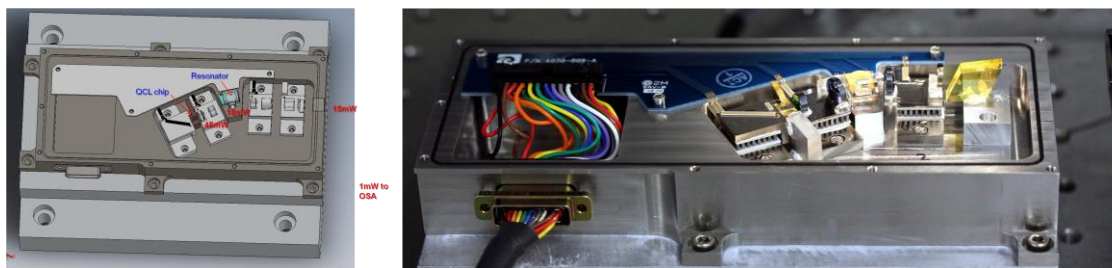
4-29: Left: Scheme of the read-board self-injection locked QCL. Right: Picture of the assembled unit.
