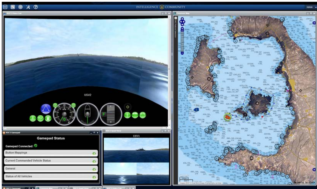
Figure 9: A screenshot of the OWF user interface display for an operator controlling a USV. The widget launched (top left to bottom right) are as follows: USV Video, Common Map, Gamepad, and Video Quad View.
