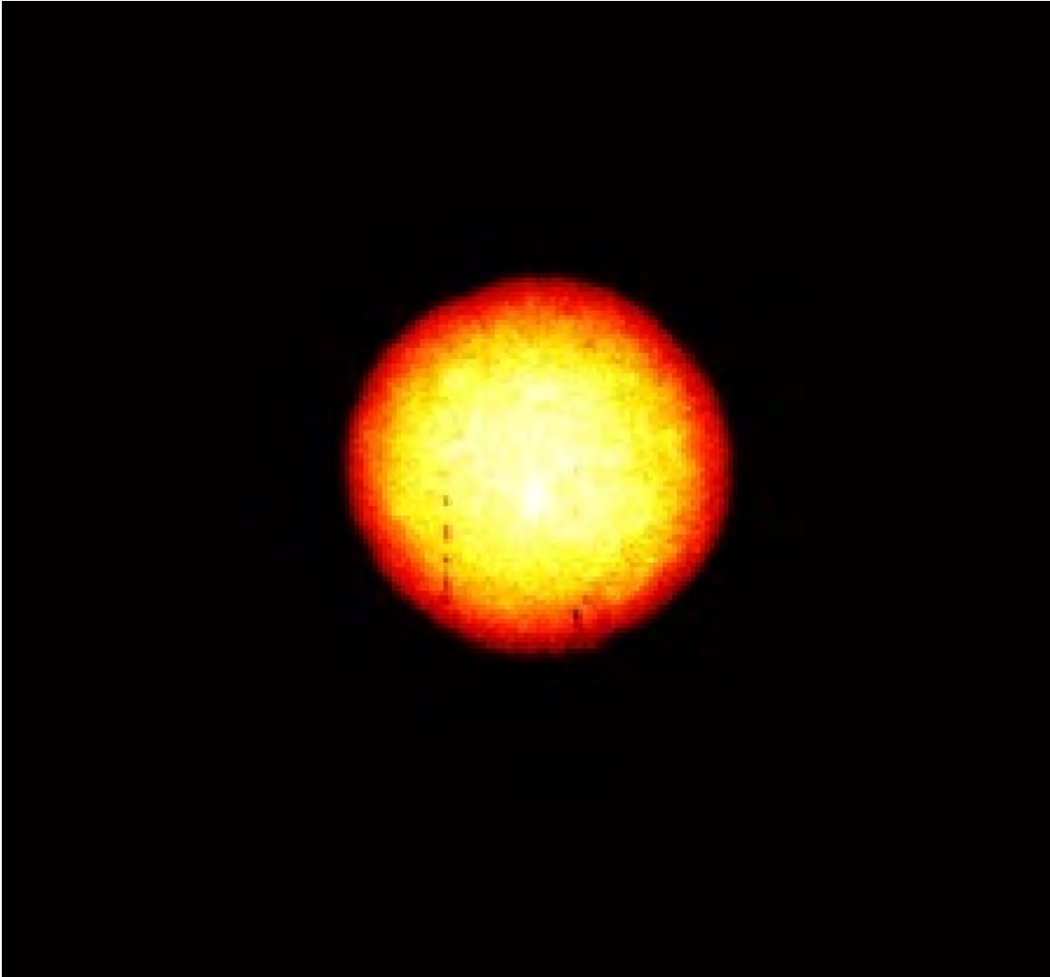
Figure 30. Non-Lambertian limb-darkening effects for event Wasp Prime. The outer edges appear cooler (red) while the center appears hotter (white). A Lambertian source would appear uniform in brightness to an observer.
