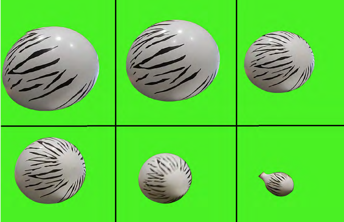
Figure 63. Six frames of a balloon used to test whether or not the fundamental null hypothesis could be used to time align separate cameras.
