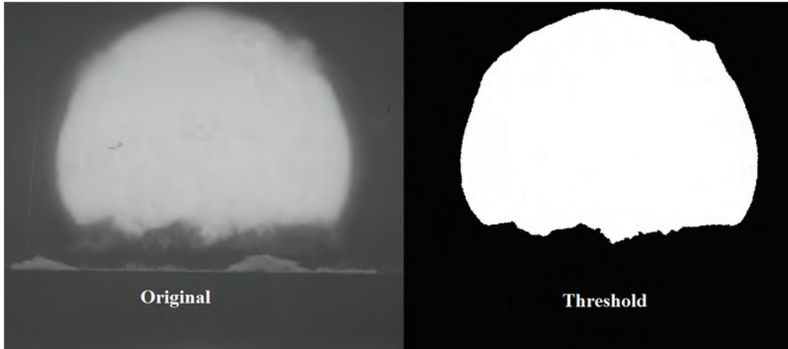
Figure 18. Example of applying an intensity threshold to an image to define the fireball region of a nuclear detonation.
