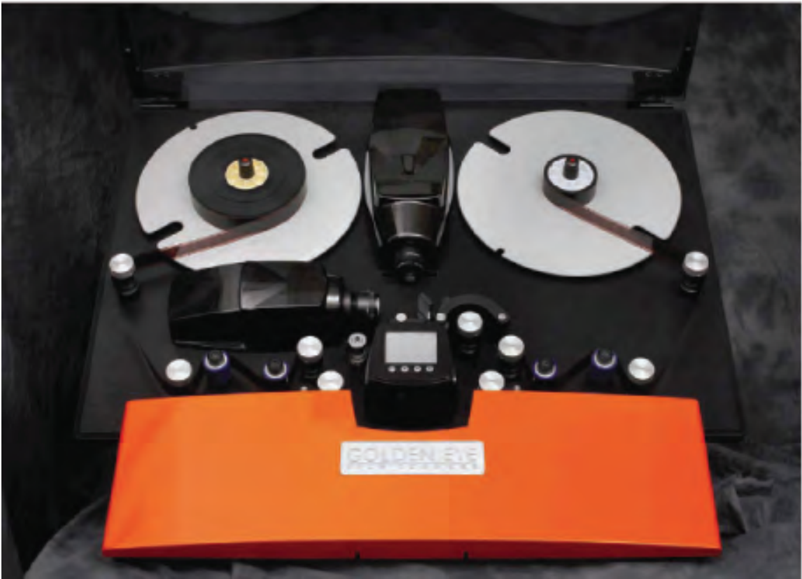
Figure 2. The Golden-Eye scanner used by LLNL to digitize nuclear testing films [11].
