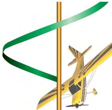
**Figure 1: Helical Flight Path of a Spin**
