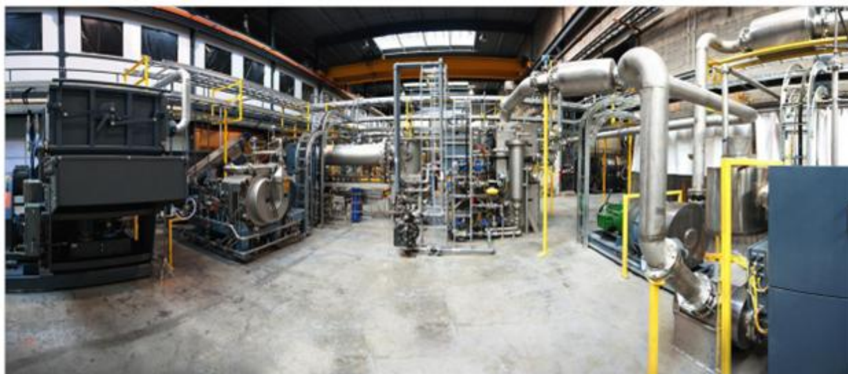
Figure 4. PAWDS for USS Gerald R. Ford supercarrier undergoing factory acceptance testing in Montreal.
