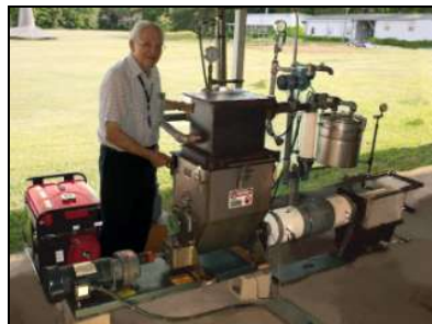
Green Liquid & Gas Technologies Indirectly Heated Gasifier
