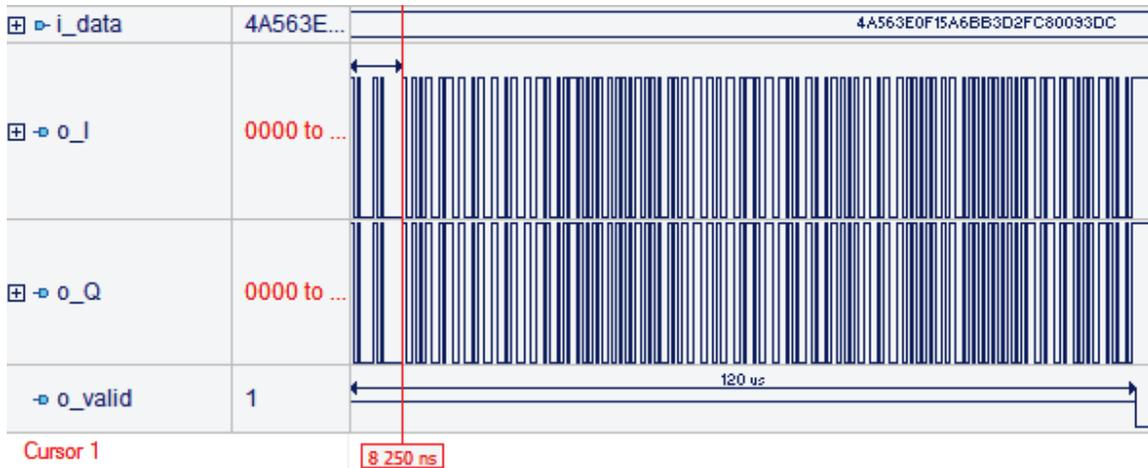
Figure 38. Screenshot of full modulation signal in Active-HDL®.
