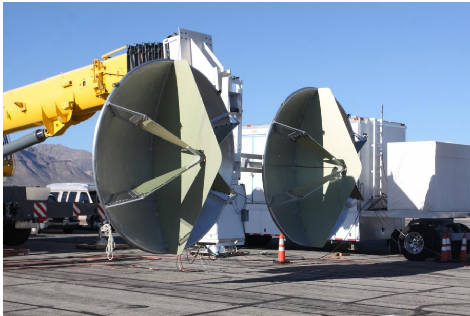
Figure 1.2. 12-foot reflector IRAs built by Farr Fields LC for the NRTF.
