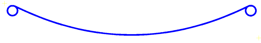
Figure 3.6. Reflector cross-section. The reflector is modeled with a perfectly smooth transition from the parabolic surface to a circular rolled edge.
