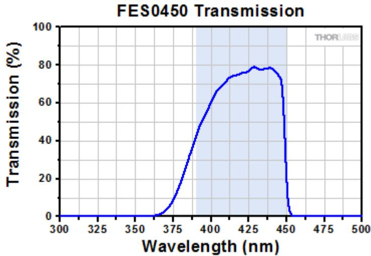
Fig. 3 Spectral characteristics of the 450-nm shortpass filter
