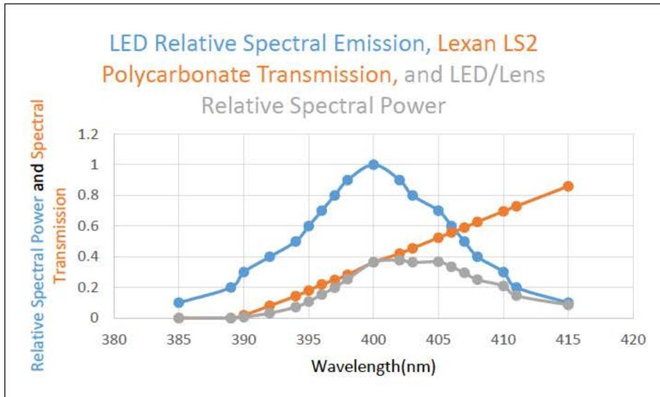
**Fig. 1 Transmission of Lexan LS2 polycarbonate near 400 nm**
