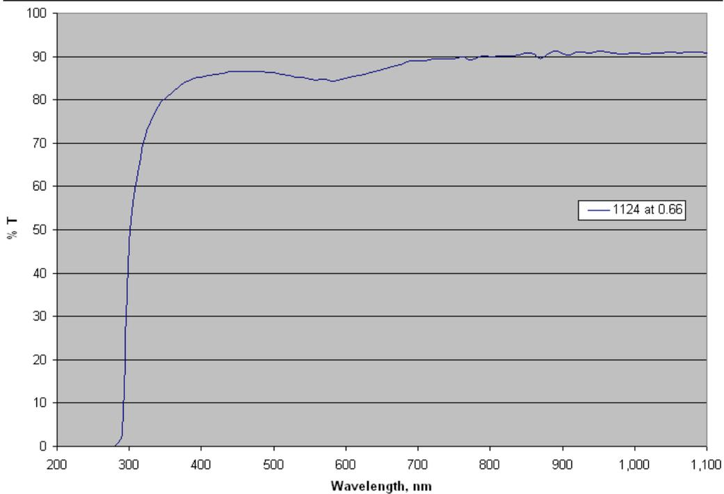
**Fig. 6** Transmission characteristics of Lexan 1125
