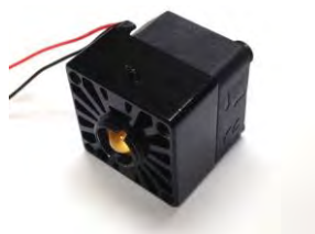
Figure 5: Reduced size LED emitter assembly with 5 mm LED, heat sink, and fan.
