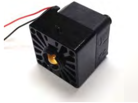
Figure 4: Reduced size LED emitter assembly with 5 mm LED, heat sink, and fan.
