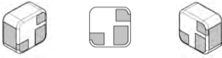
Figure 1. Plasma-shell with three-electrode pattern.
