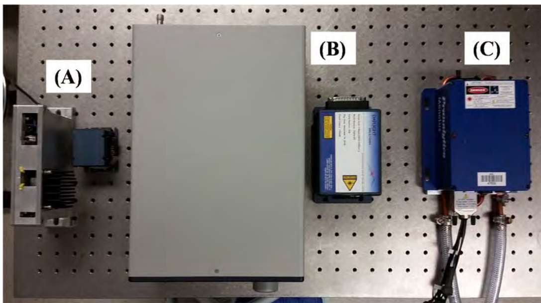
Figure 8. Photograph showing a size-by-size comparison of the various evaluated laser systems. (A) Daylight Solutions ultracompact SpriteIR pulsed EC-QCL system (laser and controller); (B) Daylight Solutions pulsed/modulated CW EC-QCL system (laser and controller); (C) Pranalytica QCW EC-QCL system (complete).
