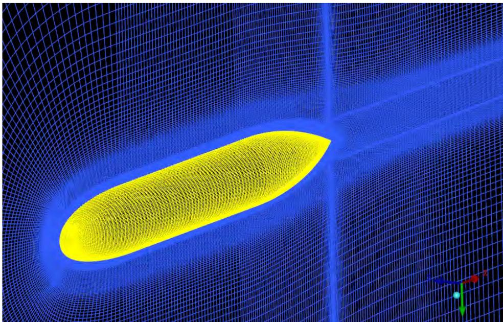
Figure 2: Detailed view of the mesh on the hull surface and the symmetry plane for the DSTO generic conventional scale model submarine.
