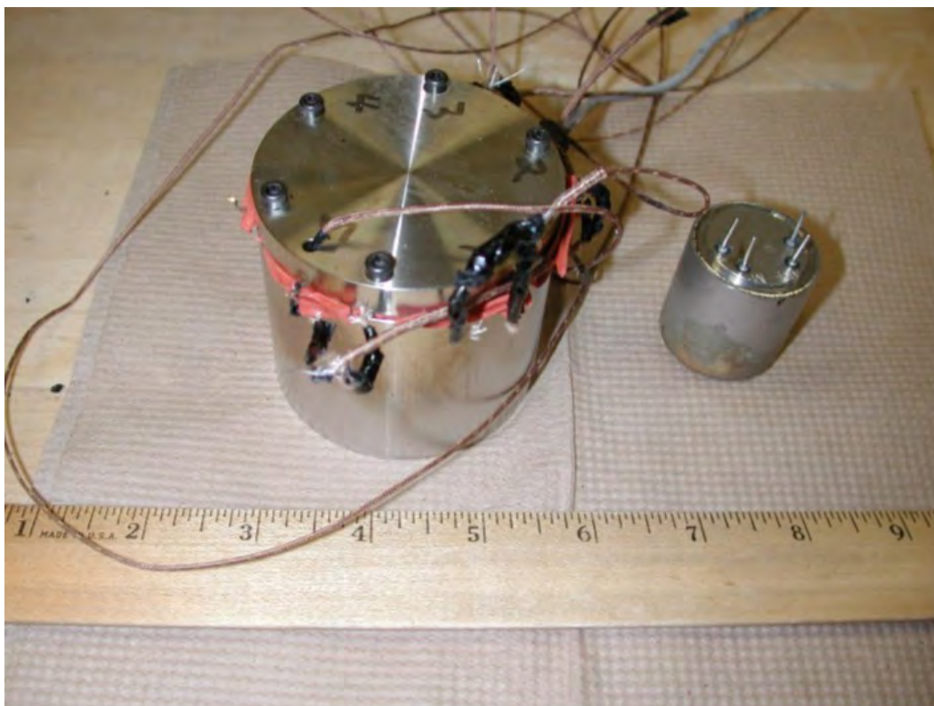
Fig. 26 LCCM thermal battery cases: thick-walled SS laboratory test fixture (left) and thin-walled SS flight case (right)
