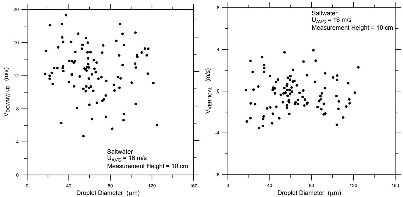
**Figure 1:** Plot of droplet velocity (m/s) versus droplet diameter in micrometers from the Spray Production and Dynamics Experiment data set. The left hand panel shows the horizontal downstream velocity plotted versus droplet diameter and the right-hand panel shows the vertical velocity plotted versus droplet diameter.
